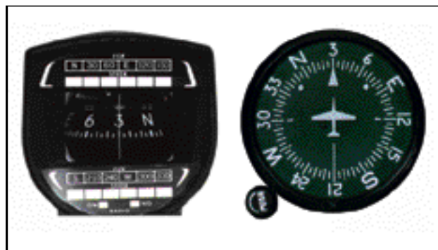
Figure 4-26. Setting the heading indicator.
