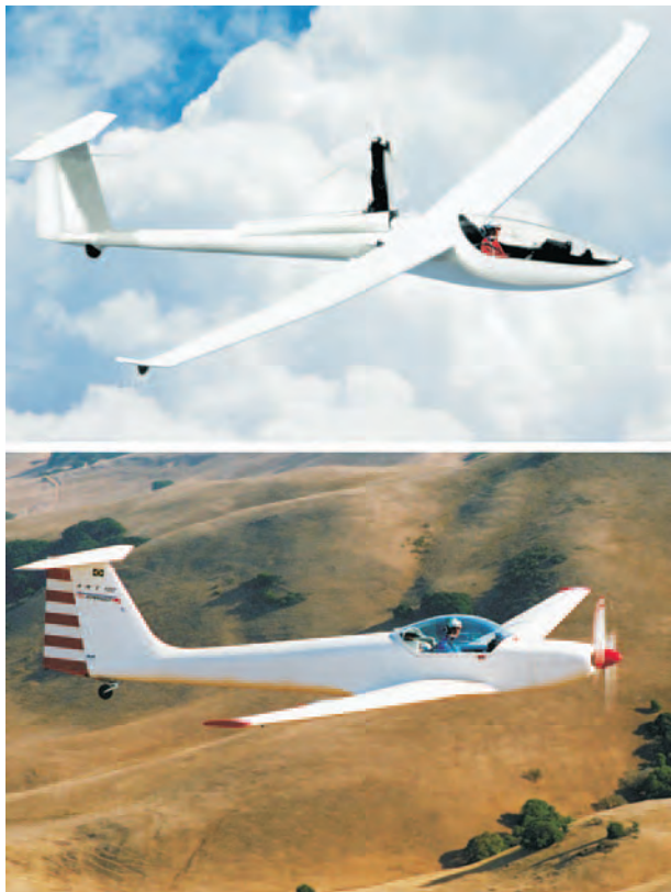
Figure 7-24. Types of self-launch gliders.
