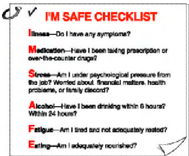
Figure 1-6. Prior to flight, you should assess your fitness, just as you evaluate the aircraft's airworthiness.
